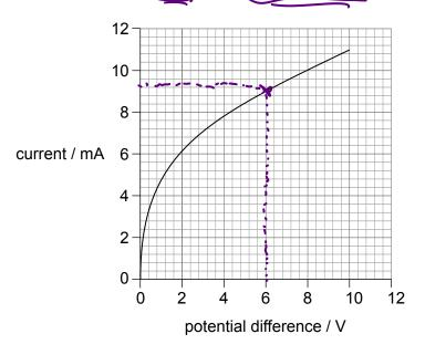
What is the resistance of the filament when the potential difference across it is 6.0 V?
