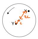
Point X is a distance <u>2L</u> from the centre of the disc. Point Y is a distance <u>L</u> from the centre of the disc. Point Y has a linear speed *v* and a centripetal acceleration *a*.
