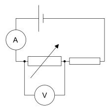
What changes occur in the ammeter reading and in the <u>voltmeter reading</u> when the resistance of the variable resistor is increased?
