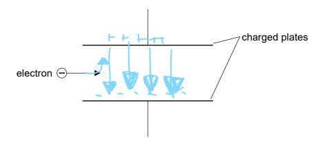
The electromagnetic force acting on the electron
